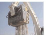
and is able to crush material from 20 to 100 mm; contains a load bucket opening of 600 x 450 mm; length of 1800 mm, width of 1050 mm and height of 1200 mm.
