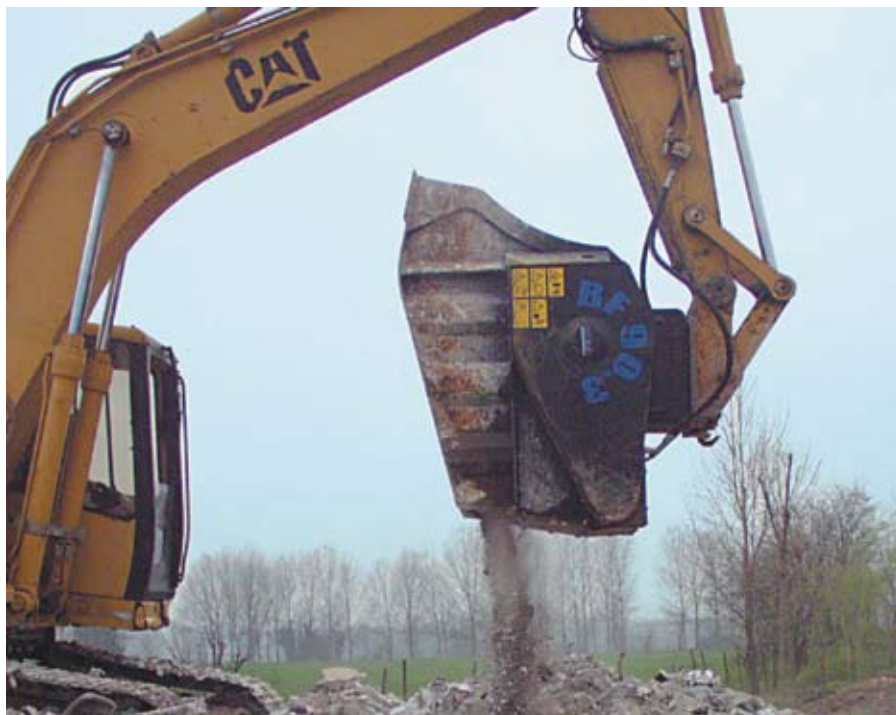
The BF90.3 bucket crusher is suitable for excavators between 20 and 28 tons.
