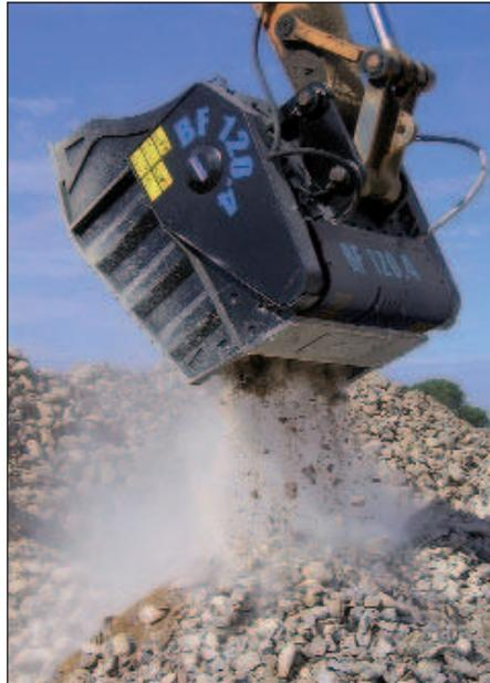
layer in road subgrade. One of the features the customer particularly appreciates is the machine's autonomy in that it needs no support equipment, although the client explained that in a quarry, it is coupled with a separating screen because sizes must be divided.
