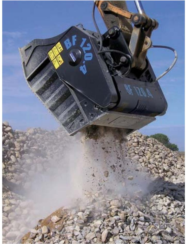
They visited the recycling site of their client, where demolition rubble from multiple sites together with excavation material and materials from natural rock quarries, are brought here for processing. The use of the bucket crusher has made the complete recovery of demolition material possible. For instance, this material, which was once taken to dumps, is extremely valuable in the road sector.
