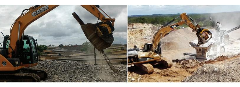
way where concrete can be separated from the iron. To facilitate this operation the suggestion is to load the bucket with an MB grapple and let the jaw and gravity do the rest. Alternatively, skilled operators can feed the bucket manoeuvring the excavator; a magnetic kit installed can also facilitate the separation and salvaging the metal.
