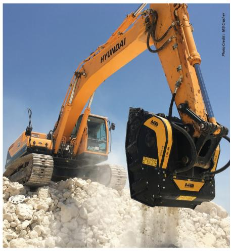
MB offers the widest range of crusher buckets, 12 models from the smallest, for mini excavators, a special range dedicated to wheel loaders, skid steer loaders and backhoe loaders, to the largest suitable for excavators from 70 tonnes and more.
