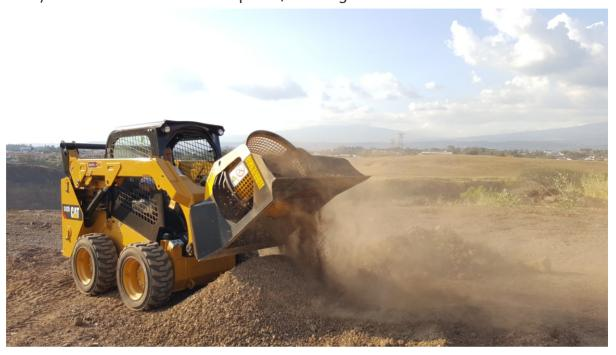
Until recently, nobody had thought of this. Then along came MB Crusher, who designed and produced machinery that transforms loaders, skid loaders and backhoe loaders into mobile crushing and screening tools.
