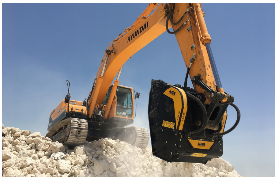
A Crusher Bucket by MB Crusher, model BF90.3 mounted on Hyundai excavator, operating in a quarry.
