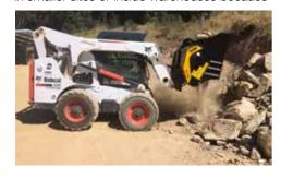
the MB-L and MB-S models are compact and easy-to-use; they are environmentallyfriendly because waste material is recycled on-site, reducing transportation to landfill and therefore vehicle pollution.
