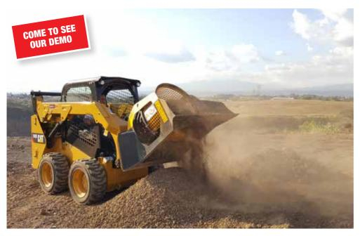
Until recently, nobody had thought of this. Then along came MB Crusher, who designed and produced machinery that transforms loaders, skid loaders and backhoe loaders into mobile crushing and screening tools.
