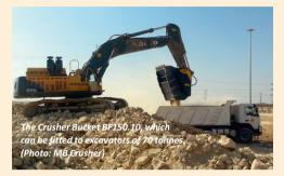
MB crusher uses exclusive and patented Made in Italy technology and is built to process all extracted material, in order to render it re-usable directly onsite. The precision of production aims to allow material that were previously destined solely for disposal to be processed in calibrated batches, which can be re-sold or re-used on-site, thus leaving the mineral balance of the quarry unaltered.
