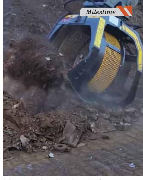
MB Crusher screening bucket can quickly select any material that is homogeneous in size.
