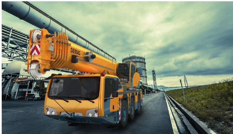
■ The AC 60-3 has a 50m main boom and can be fitted with a 16m extension, for the longest configuration in its class.
