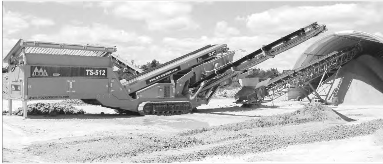
IROCK's two-deck TS-512 portable tracked screening plant offers hassle-free setup and portability.
