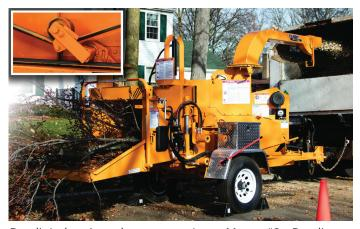
Bandit Industries sales manager Jason Morey. "On Bandit clutchless hand-fed chippers, damage from improper use is typically limited to the main drive belt, which is far easier and less expensive to maintain or replace than a clutch."
