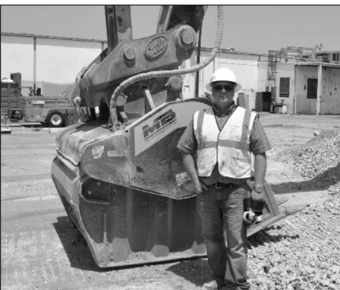
*Using this attachment, Keith Randall was able to reduce the concrete to -3 in. size on site and recycle the crushed material as fill around the new footings that were to be poured.*
