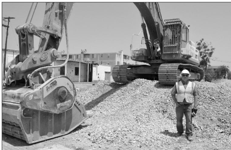
*The BF 120.4 is designed for large demolition jobs, crushing in quarries and aggregate recycling to reduce the volume of materials.*
