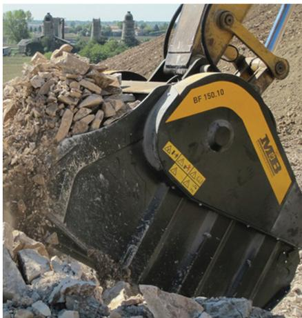
This year MB presented two gems: the BF 150, with its 10 tonnes of weight and title of biggest bucket in the world, and the MB-L, the smallest crusher made by the company.
