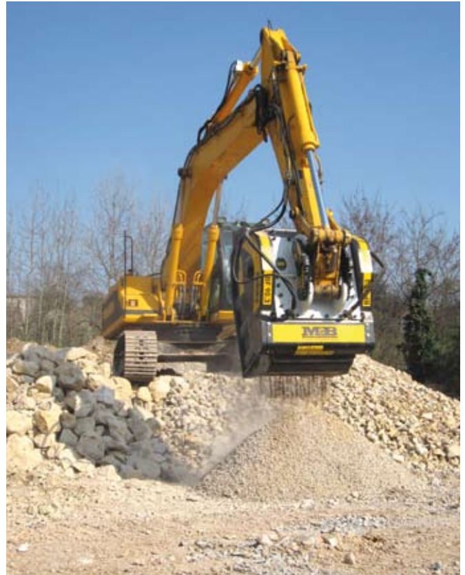
MB crusher bucket is very useful during excavation and filling jobs. It is also easy to transport and has low maintenance costs.
