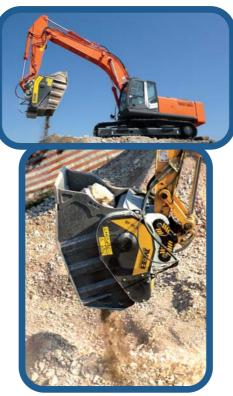
Special attention should also be paid to the crusher bucket being employed to crush inert materials to be subsequently used to form the stabilized pavement
