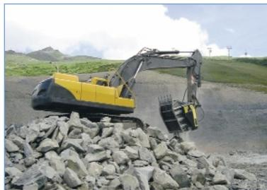
the material and producing the stabilized pavement directly on site, thereby saving time and reducing costs. Tokyo has one of the most expensive transportation systems in the world, and trucks are forced to make many trips to complete a job. One problem that MB effectively solves since materials are crushed on site and consequently there is no need to transport them to another location.
