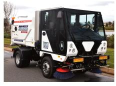
the capability of a greater work rate thanks to its greater road speed of 65 km/h, hydrostatic drive system, compact dimensions, generous payload capacity, a large water tank and also its strong chassis.
