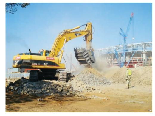
Jaw-action bucket crushers by MB are used in mobile excavators for many construction and building operations including roadwork, excavation, demolition, quarries and mines. The product line covers an excavator range from 8 to more than 28 tons.
