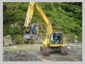
The BF90.3 bucket crusher attached on a Komatsu excavator.
