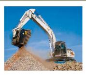
and economical. The crusher bucket is available in four versions: BF60.1 (suitable for excavators weighing 8 to 14 tons), BF70.2 (suitable for excavators of 14 to 20 tons), BF90.3 (suitable for excavators of 20 to
