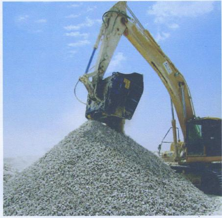
The MB bucket crusher was the first of its kind. It operates by utilising the hydraulic system of the excavator on which it is installed and is available for a wide range of excavators from 8t upwards.
