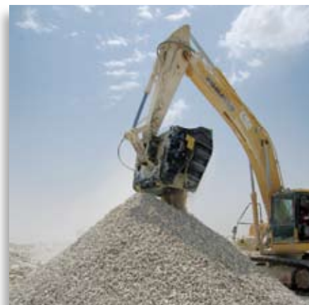
A MB BF120.4 bucket crusher, attached to a Komatsu machine, feeds the stockpile.
