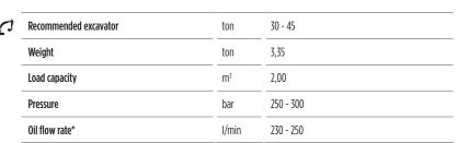
$<sup>^{\</sup>ast}$  The minimum hydraulic flow rate value must be alongside the required operating pressure.
