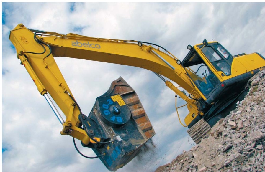
Unlike a conventional crusher, a bucket crusher is operated by hydraulic power provided by the excavator on which it is installed, with which it functions in synergy.
