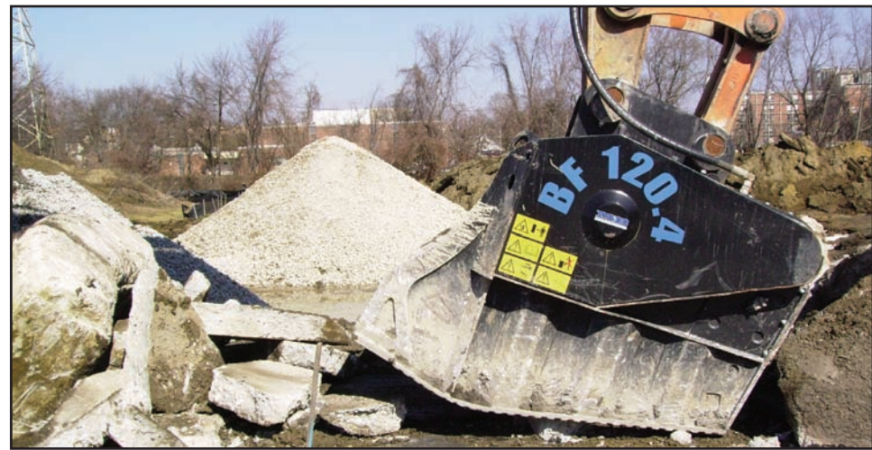
The Eco-Crusher jaw crusher bucket recycles up to 15-inch minus material.
