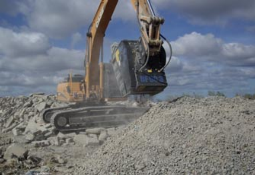
The MB Crusher Bucket can crush material down to between 20mm and 120mm
