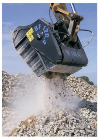
BF 120.4 The machine weighs 4.9t and is recommended for excavators weighing upto 28t. Material measuring up to 120 by 45cm and about 1m3 in size, can be crushed at one time. The size of the crushed material can be adjusted to between 20 and 120mm. Hourly production rate is between 25 and 50m<sup>3</sup>.
