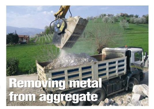
Increased versatility will be offered by MB Crusher as the firm now offers a magnetic separation option for its excavator-mounted bucket crushers
