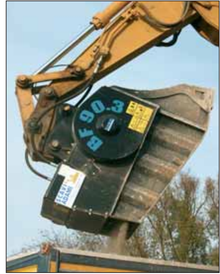
■ La geometria delle mascelle interne tende ad accompagnare il materiale piuttosto che solo a comprimerlo The geometry of the internal jaws tends to feed the material through as opposed to just compressing it
