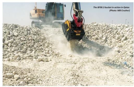
texture, thicknesses can be added into or removed from the MB crusher in just a few minutes. The crushed rock will be reused to fill on-site excavations and as subgrade for the roads within the school.
