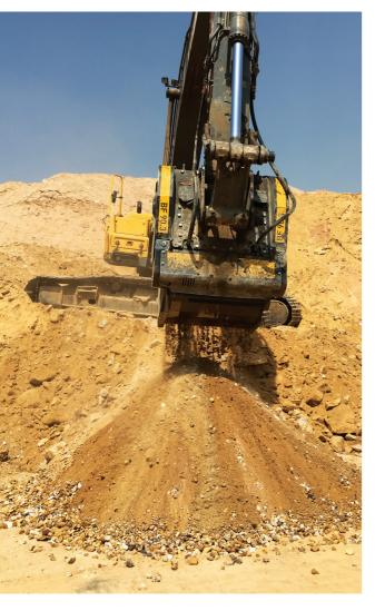
However, due to MB Crusher's robust construction, this is not as high a concern as it can be. The jaws and blades of MB Crushers are made of the finest grade Hardox steel – one of the toughest material known to man, he adds. Despite this, should any problem arise, Amtrac is on hand to lend full support.
