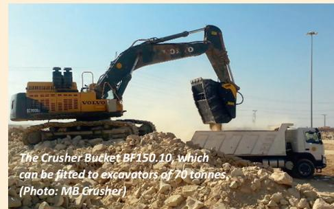
The Crusher Bucket BF150.10, which can be fitted to excavators of 70 tonnes. (Photo: MB Crusher)
