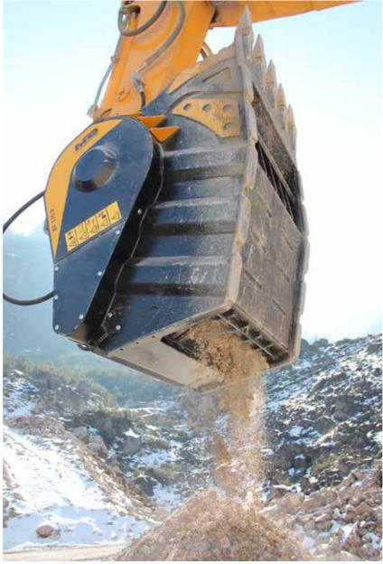
Crusher and screening buckets allow operators and contractors to reprocess materials in situ, helping reduce the load on the environment by making useful by-products of otherwise low value raw feed, which may add significantly to their profitability. In urban areas the carting and dumping costs alone often mean a fast ROI, and in rural areas it can mean producing very useful and valuable materials in places where buying materials is often prohibitively expensive.
