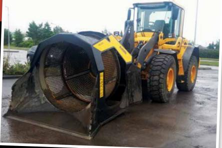
The MB-LS 220 is the latest and largest in MB's LS series of mobile screening buckets. The series has two more models, the smaller of which is the MB-LS 140, suitable for skid steer loaders and backhoe loaders from 2.6t, and the MB-LS 170, which is designed for skid steer loaders and backhoe loaders from 6.5 to 11t.
