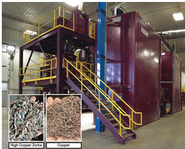
Ohio-based Best Process Solutions, Inc. (BPS) is seeing the results of the first installation of the company's RecoverMax Fines Process. While many companies separate metal pieces that are ½-inch or more in size, this technology is designed to handle smaller fractions. According to
