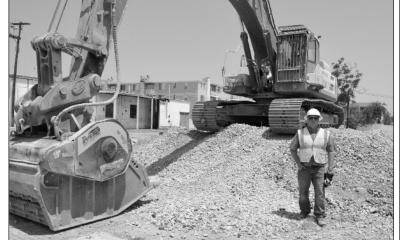
The BF 120.4 is designed for large demolition jobs, crushing in quarries and aggregate recycling to reduce the volume of materials.
